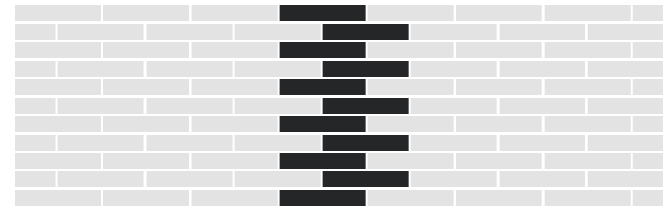
Stretching bond half stone moved
